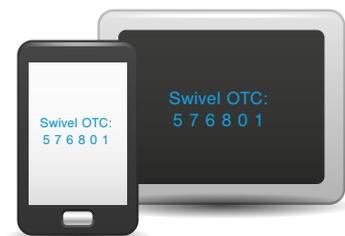
Swivel is a tokenless two-factor and strong authentication platform that authenticates users via its one-time-code (OTC) extraction protocol, PINsafe. The OTC is extracted from a security string, which is delivered to the user via a variety of methods (in this instance, Tullow Oil is using SMS), which eliminates the need for tokens.
